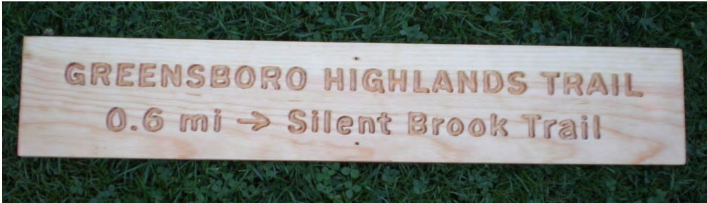
Figure 4: Wooden Routed Sign - Franklin Gothic FONT size 110 bold (approx. 1 1/8" letters) cut with plunge router using 1/4" round-nose bit
